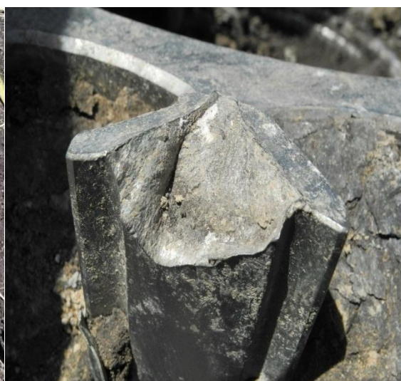
FIGURE 39: R/H ENGINE - S/N 602695 - RETENTION LUGS - FRACTURED
