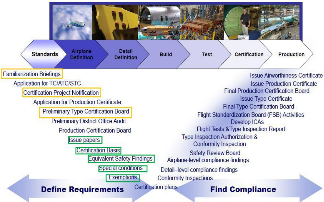
FIGURE 79: DIAGRAM OF FAA CERTIFICATION PROCESS
