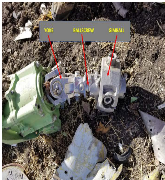
FIGURE45: FLAP TRANSMISSION &amp; BALLSCREW
