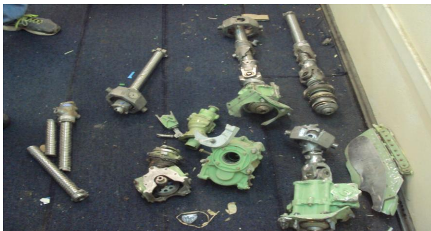
FIGURE47: TRAILING EDGE FLAP TRANSMISSIONS AND BALL SCREWS
