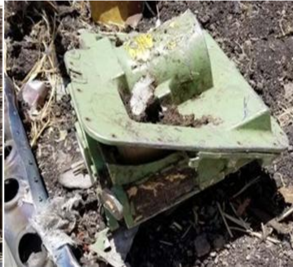
FIGURE 51:STAB TRIM ELECTRIC MOTOR HOUSING
