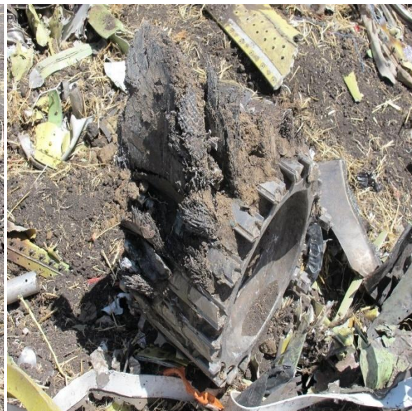
FIGURE 37: - R/H ENGINE - S/N 602695 - FAN DISK
