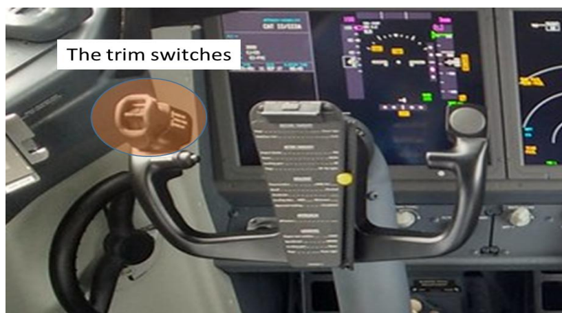
FIGURE 11: TRIM SWITCHES ON THE LH YOKE
