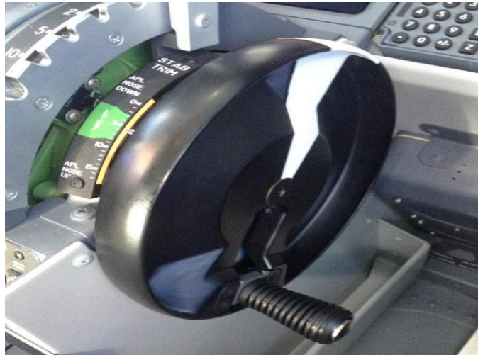
FIGURE 12: THE TRIM WHEEL, WITH THE HANDLE EXTENDED
