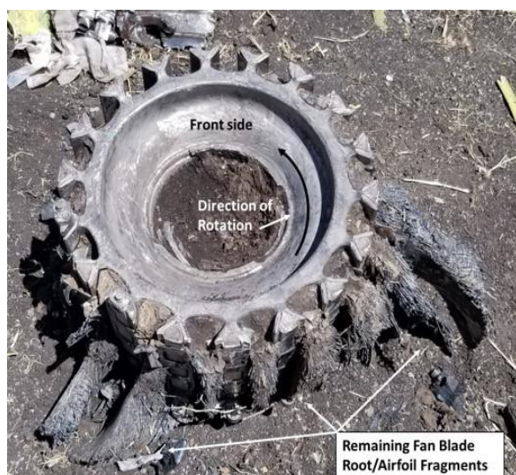
FIGURE 38: R/H ENGINE - S/N 602695 - FAN DISK
